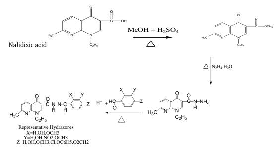
Scheme 1: Basic scheme for preparation of hydrazones from nalidixic acid
