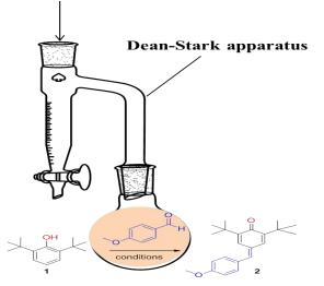
**Fig. 1:** Synthesis of 2,6-di-*tert*-butyl-4-(4-methoxybenzylidene)cyclohexa-2,5-dienone using Dean Stark apparatus
