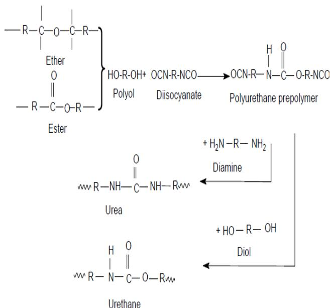
**Fig. 1:** Chemical reactions involved in polyurethane synthesis
