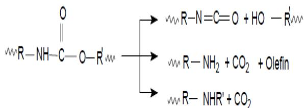
**Fig. 3:** Thermal degradation of urethane linkage
