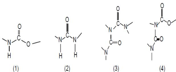
**Fig. 2:** Chemical structures of different isocyanates linkages (1. Urethane 2. Urea 3. Biuret 4. Allophanate)
