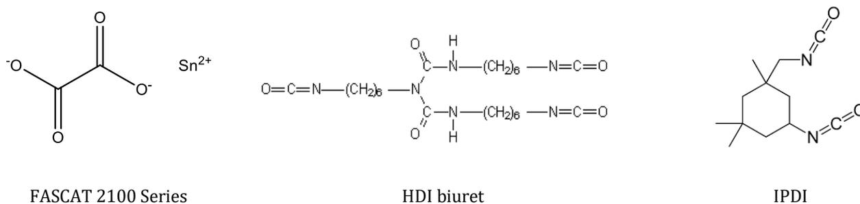
Fig. 4: Chemical structures of FASCAT 2100 Series/HDI biuret/IPDI
