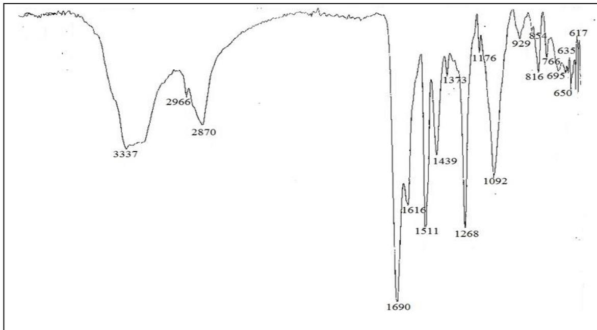
**Fig. 5:** ATR spectrum of conventional aminolysed product using EDA
