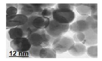
Fig. 3: TEM image of CuO NPs synthesized using flowers aqueous extract of Bougainvillea
