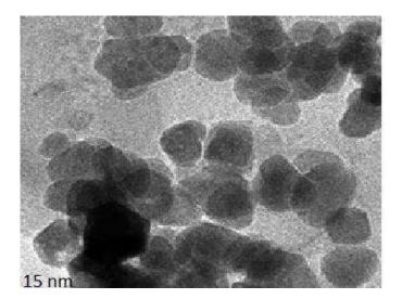
**Fig. 5:** TEM of green synthesize CuONPs by *Bougainvillea* leaves aqueous extract
