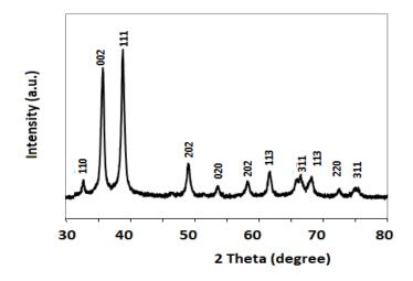
**Fig. 2:** XRD pattern of green synthesized CuONPs by *Bougainvillea* leaves aqueous extract
