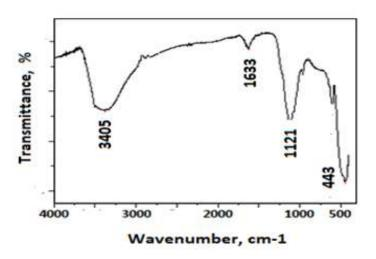
Fig. 4. FT-IR analysis of green synthesized CuONPs
