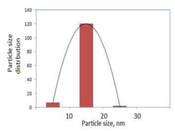
**Fig. 6:** Particle size distribution histogram of synthesized CuONPs
