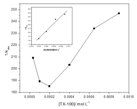
Fig. 8. Reciprocal of observed rate constant vs. TX-100 concentration at 297K and fixing other conditions.
