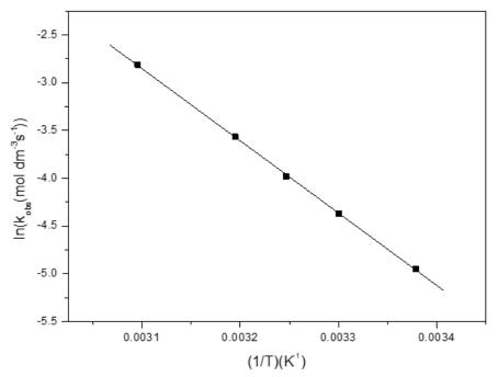
Fig. 6. logarithm of observed rate constant vs. reciprocal of temperature and fixing other conditions.
