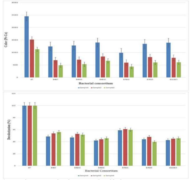
Fig. 5: Water quality parameters values after treatment, color and decolorization percentage
