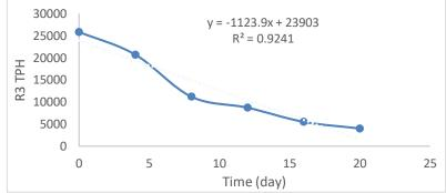
Fig. 3: TPH concentration versus time for R3 (60 g)
