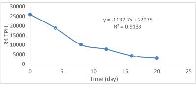
Fig. 4: TPH Concentration versus time for R4 (80 g)
