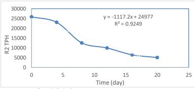
Fig. 2: TPH concentration versus time for R2 (40 g)
