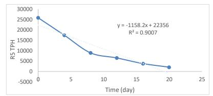
Fig. 5: TPH concentration versus time for R5 (100 g)
