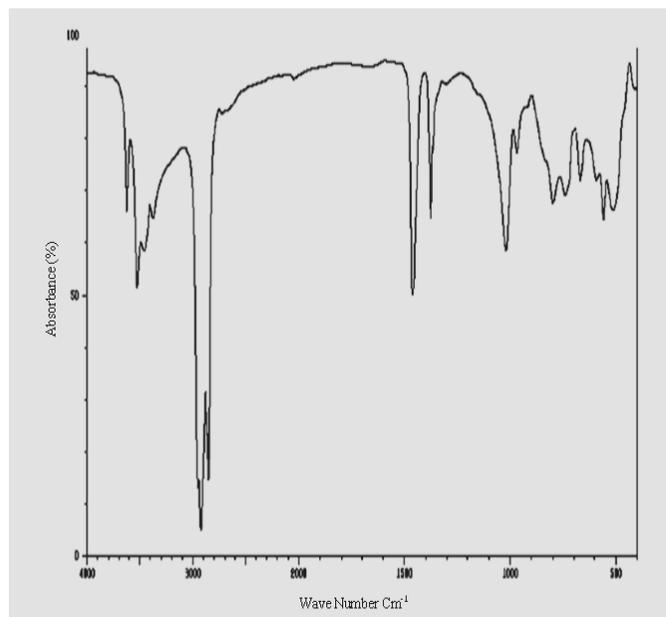
**Fig. 2:** FT-IR spectrum of aluminum hydroxide
