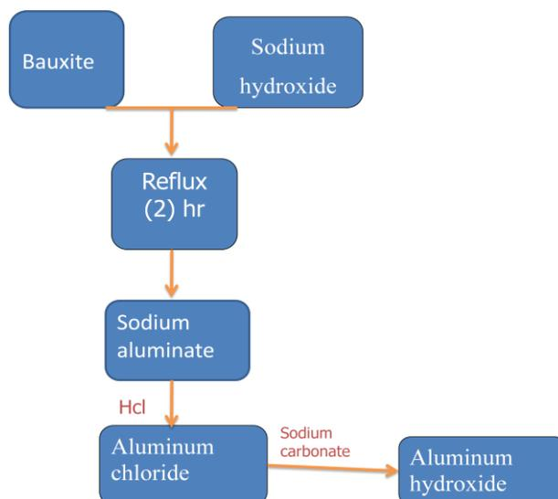
**Fig. 1:** Schematic diagram for extraction of aluminum hydroxide from bauxite
