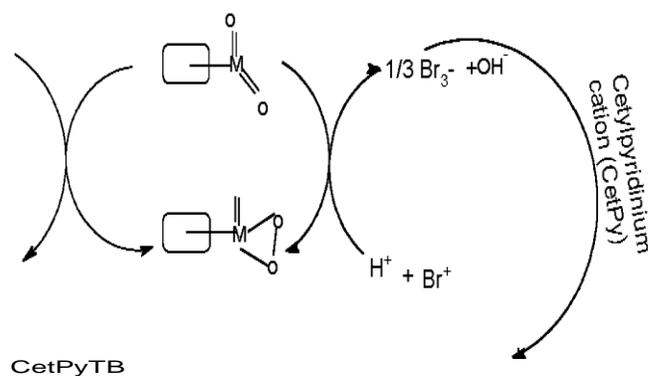
**Fig. 2:** CetylpyridiniumTribromide Synthesis Path (M = Mo and O = any ligand other than Peroxo)
