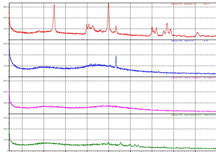
**Fig. 1:** Diffractogram, (a) kaolin, (b) obtained silica (SiO<sub>2</sub>), (c) Silica Gel, (d) H<sub>2</sub>SO<sub>4</sub>/SiO<sub>2</sub>
