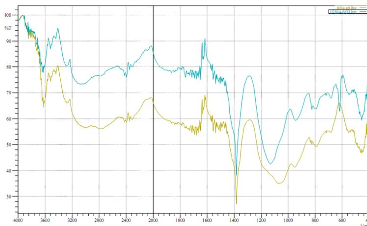
**Fig. 2:** FTIR spectra of, (a) silica gel, (b) H<sub>2</sub>SO<sub>4</sub>/SiO<sub>2</sub>
