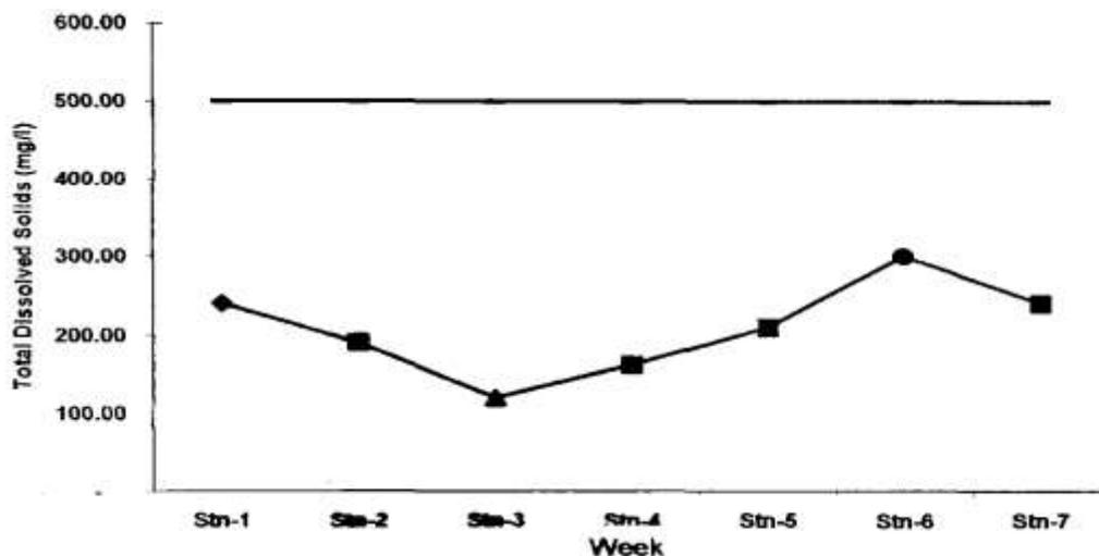
Fig. 4: Total dissolved solids (mg/l) in ground water at different stations and time
