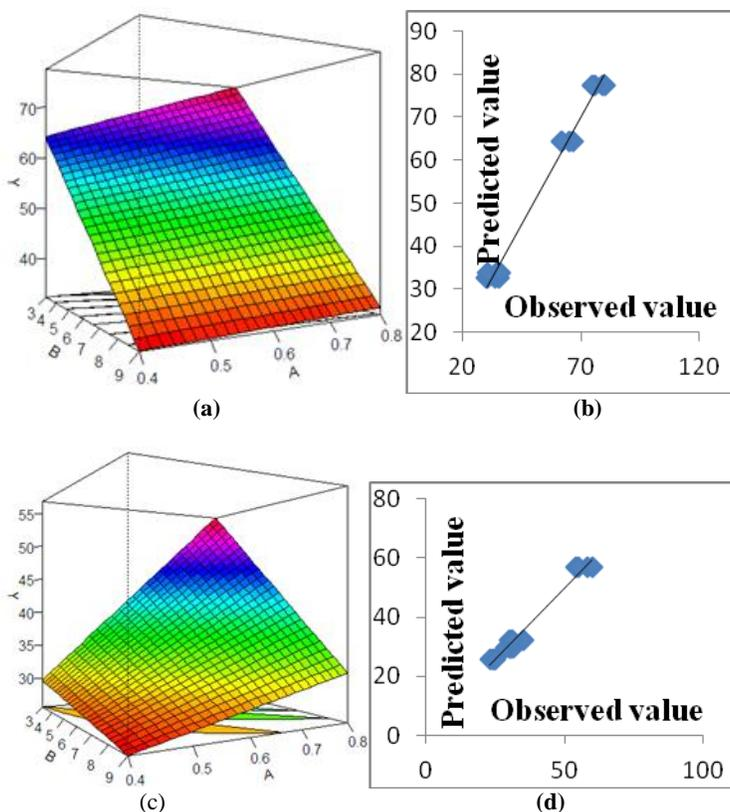
**Fig. 3:** (a) response surface (A-TiO<sub>2</sub>, B-H<sub>2</sub>O<sub>2</sub> and Y-BOD) and (b) scatter plot (observed vs. predicted values of BOD removal), (c) response surface (A-TiO<sub>2</sub>, B-H<sub>2</sub>O<sub>2</sub> and Y-DO) and (d) scatter plot (observed vs. predicted values of DO)
