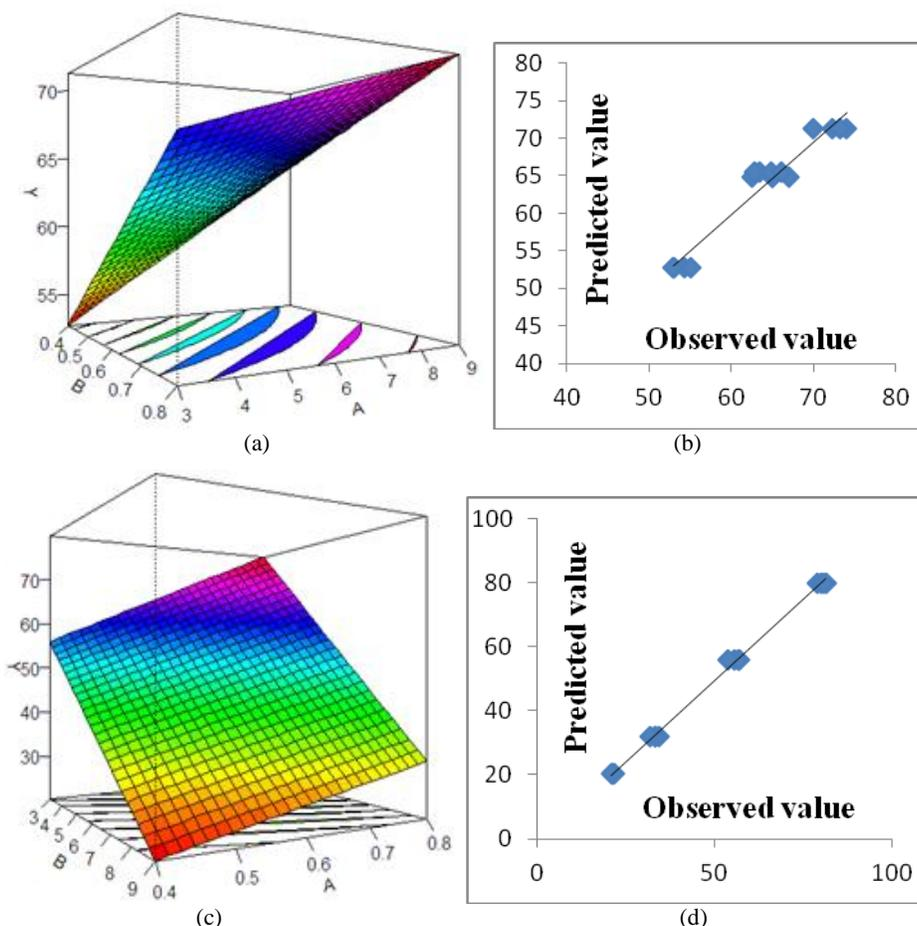
**Fig. 1:** (a) response surface (A-H<sub>2</sub>O<sub>2</sub>, B-TiO<sub>2</sub> and Y-degradation), (b) scatter plot (observed vs. predicted values), (c) response surface (A-TiO<sub>2</sub>, B-H<sub>2</sub>O<sub>2</sub> and Y-COD) and (d) scatter plot (observed vs. predicted values of COD removal)
