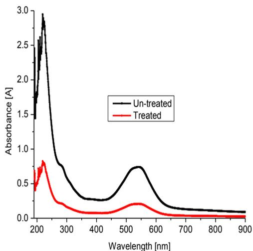
**Fig. 2:** UV-vis spectra of treated and untreated wastewater
