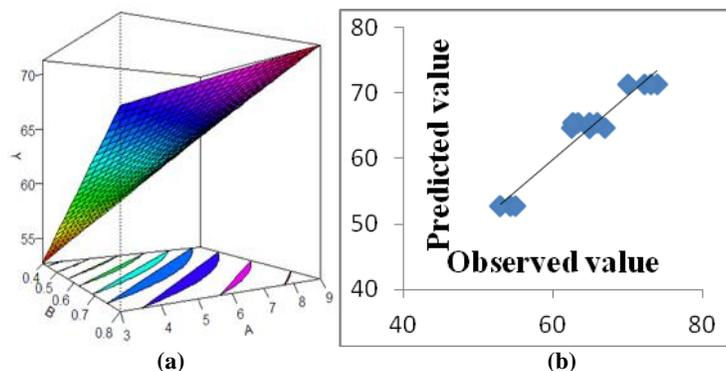
**Fig. 4:** (a) response surface (A-H<sub>2</sub>O<sub>2</sub>, B-TiO<sub>2</sub> and Y-TOC) and (b) scatter plot (observed vs. predicted values)
