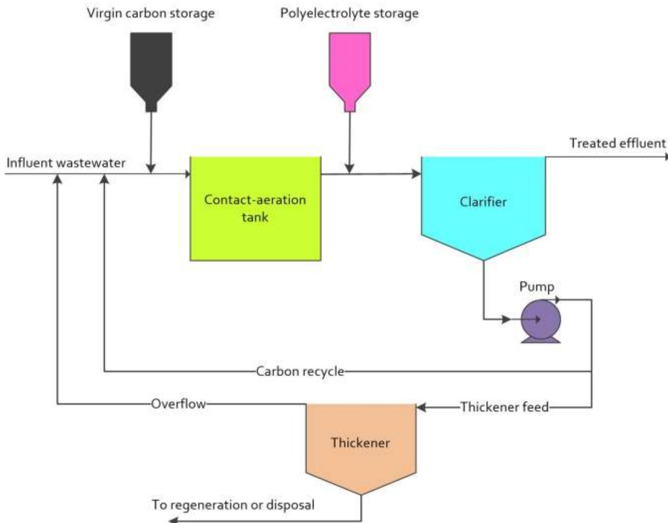
**Fig. 1:** Schematic of a typical powdered activated carbon treatment (PACT) process (modified from Meidl, 1992; 1997; IPIECA, 2010; Jafarinejad, 2017a).
