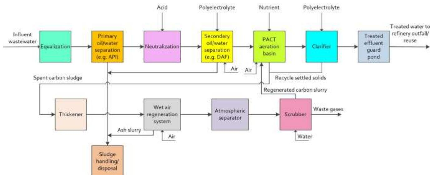
**Fig. 3:** The simplified process flow diagram (PFD) of a refinery WWTP consisting of PACT process (modified from Meidl, 1997).
