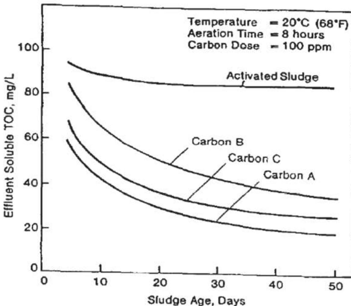
**Fig. 2:** Effect of sludge age on effluent soluble total organic carbon (TOC) in activated sludge and PACT systems (Meidl, 1997).
