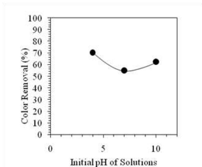
**Fig. 2:** Color removal as a function of initial pH of solutions (V sample = 500 mL; mPAC = 20 mg ; Temperature=25 ±1°C ; Agit =300 rpm ; Contact time = 1 h).
