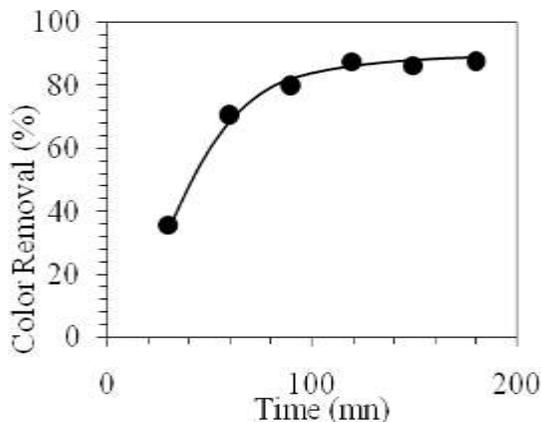
**Fig. 3:** Color removal as a function of contact time (V sample = 500 mL; pH<sub>i</sub> = 4 ± 0,05 ; m<sub>B</sub> = 20 mg ; T = 25 ± 1 °C; Agit. = 300 rpm).
