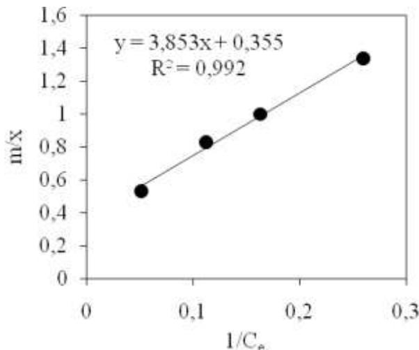
**Fig. 4:** Langmuir Adsorption isotherm of dye onto natural bentonite.
