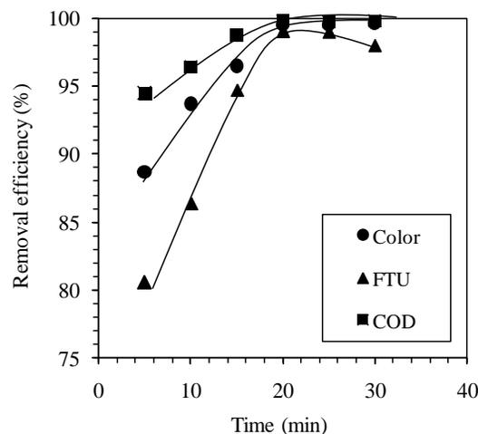
**Fig. 7:** Removal efficiency color (●), COD (■) and residual turbidity (▲).
