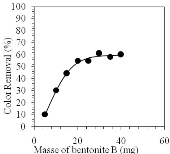
**Fig. 1:** Color removal as a function of the bentonite B masse (V sample = 500 mL ; Temperature=25 ±1°C ; pH=7± 0.05; Contact time=1 h).
