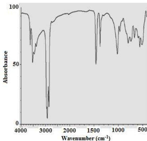
**Fig. 2:** FT-IR spectrum of aluminum hydroxide
