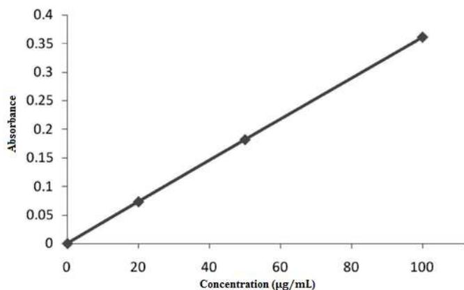
**Fig. 4:** Calibration graph for cobalt
