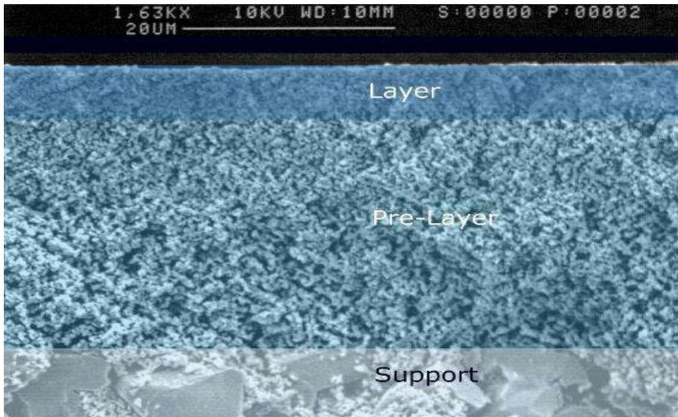
**Fig. 1:** Thin film composite polyamide membrane composition
