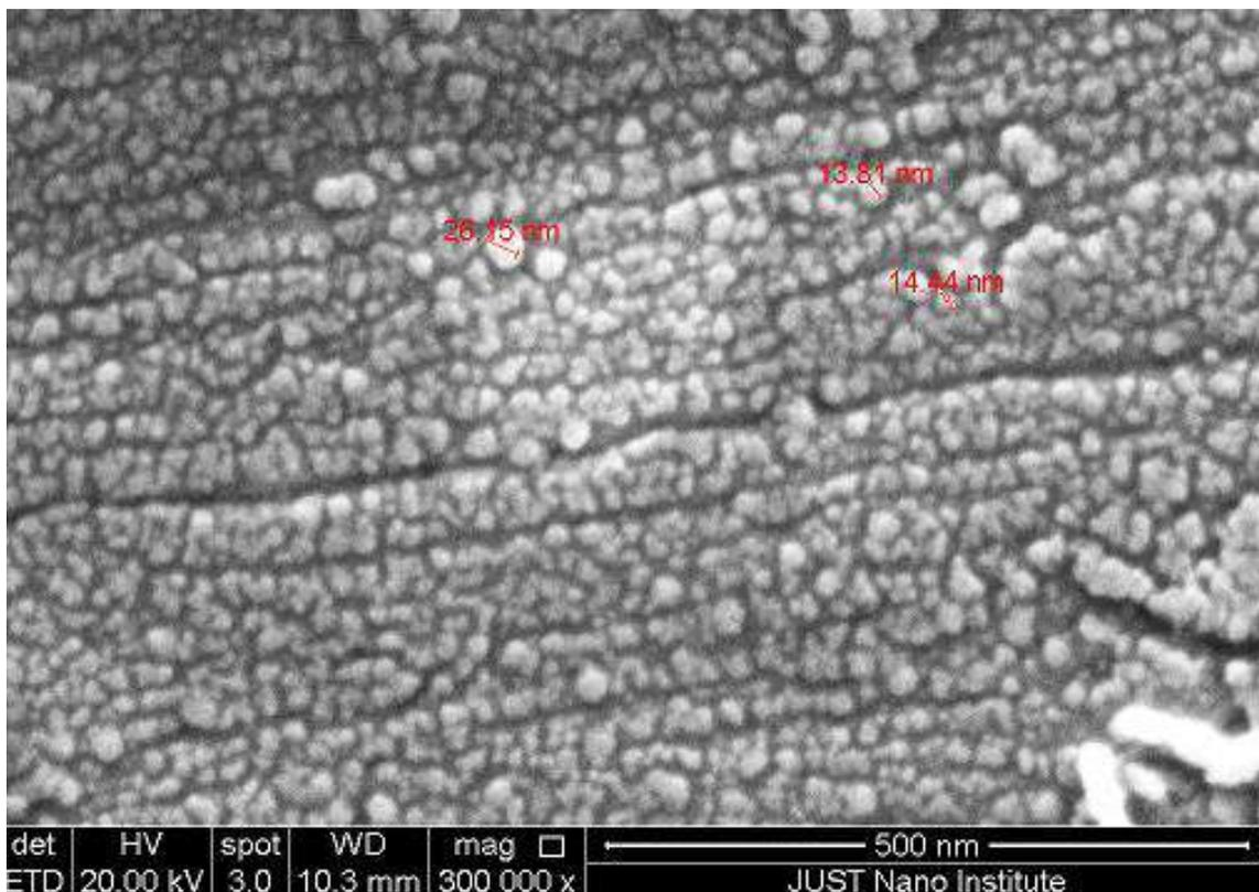
**Fig. 5:** SEM pattern of synthesized  $\text{Ag}_2\text{SNPs}$
