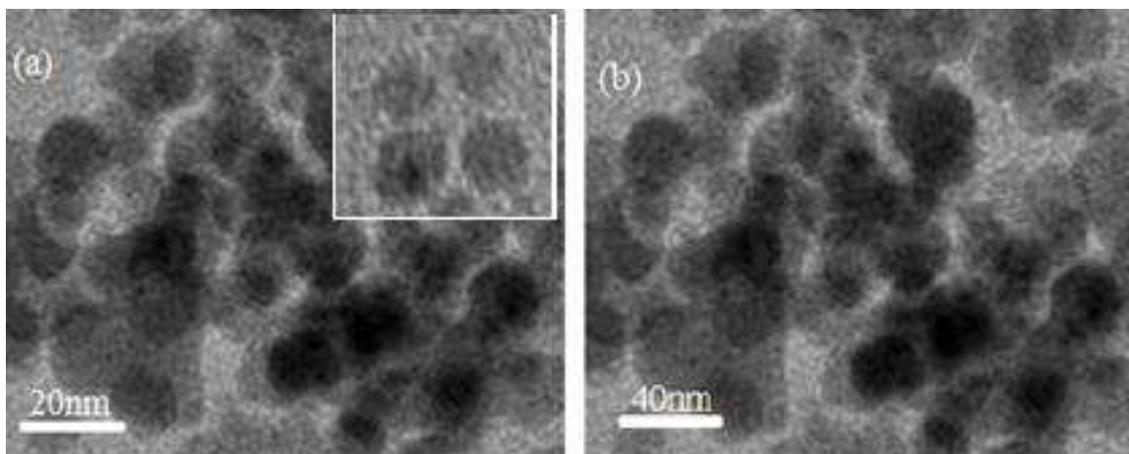
**Fig. 6:** TEM images of synthesized  $\text{Ag}_2\text{SNPs}$
