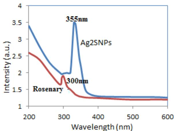
Fig. 2: UV-vis absorption spectra of silver sulfide
