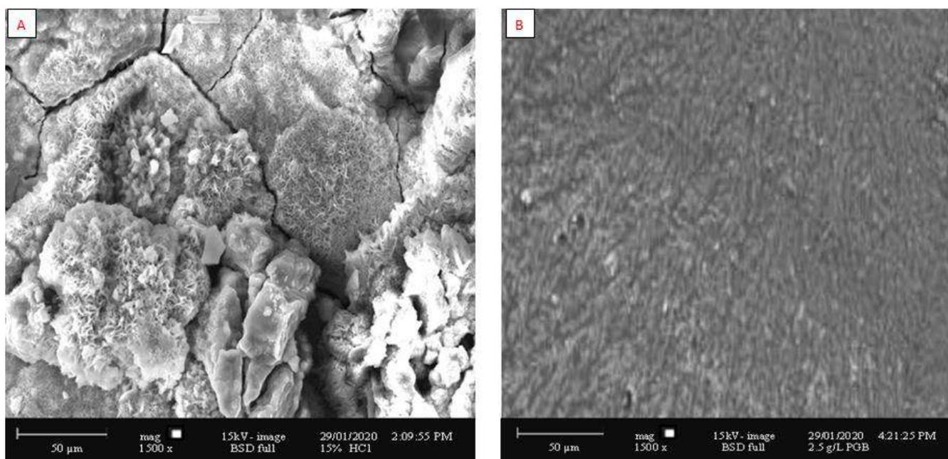
**Fig. 7:** SEM pictures of X60 steel in (a) free 15% HCl solution and (b) presence of 2.5 g/L PGB after 4 h immersion time at 303 K.
