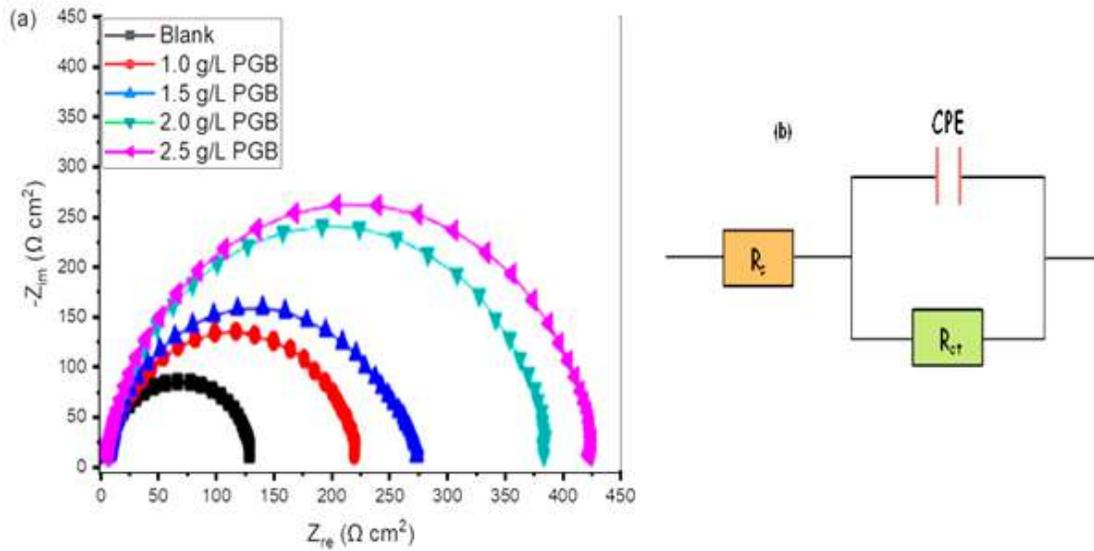
**Fig. 4:** (a) Nyquist plot of X60 steel in 15% HCl with different concentrations of PGB, (b) Equivalent circuit model used to fit Nyquist experimental data
