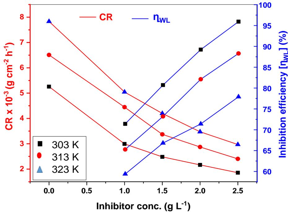
**Fig. 2:** Variation of X60 steel corrosion rate and inhibition efficiency with inhibitor concentration for PGB at different temperatures
