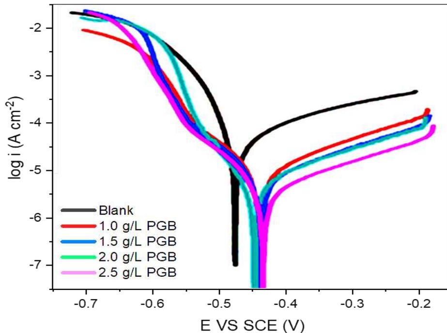
**Fig. 3:** Polarization curves for X60 steel corrosion in 15% HCl solution in the absence and presence of different concentrations of PGB
