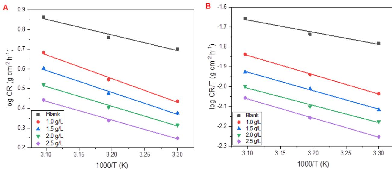
**Fig. 6:** (a) Arrhenius plots for X60 steel in 15% HCl without and with various concentrations of PGB and (b) Transition state plots for X60 steel in 15% HCl without and with various concentrations of PGB
