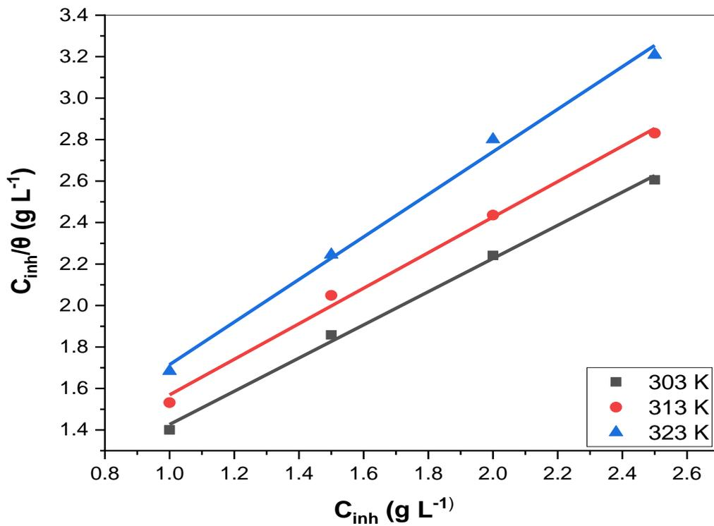
**Fig. 5:** Langmuir adsorption isotherm for PGB in 15% HCl at different temperatures
