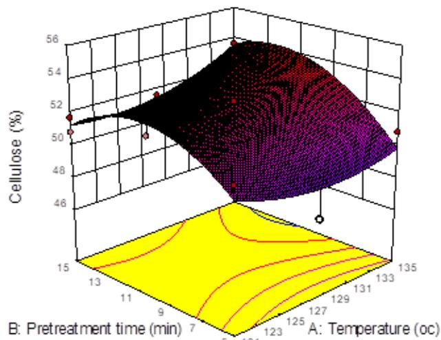
**Fig. 7:** 3D for the interaction effect of temperature and pretreatment time on cellulose content after hot water pretreatment
