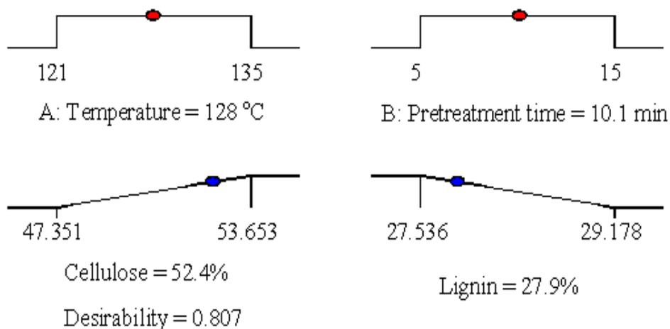
**Fig. 9:** Ramp plot of optimization solution for the responses
