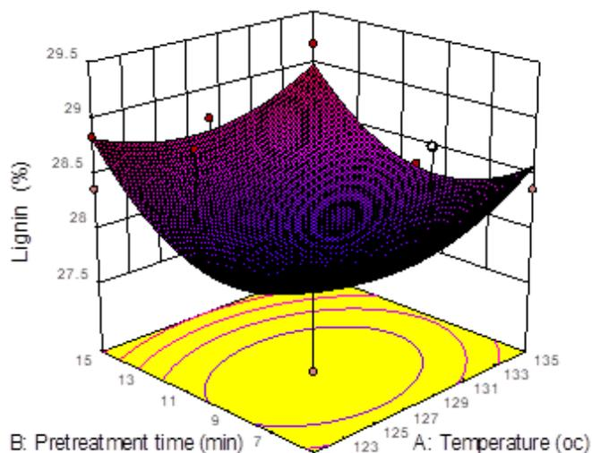
**Fig. 8:** 3D for the interaction effect of temperature and pretreatment time on lignin content after hot water pretreatment
