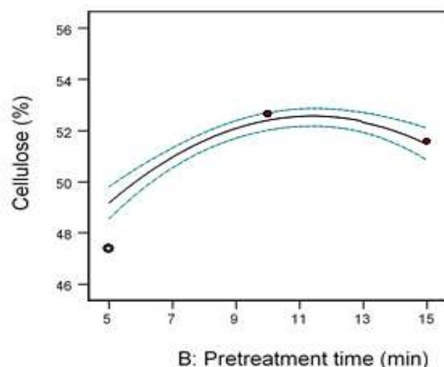
Fig. 3: Effect of pretreatment time on the cellulose content after hot water pretreatment
