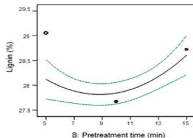
Fig. 6: Effect of pretreatment time on lignin after hot water pretreatment
