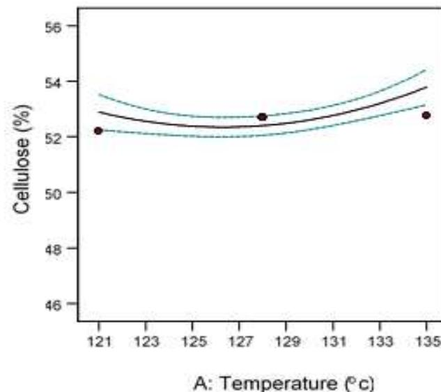
Fig. 4: Effect of temperature on cellulose content after hot water pretreatment
