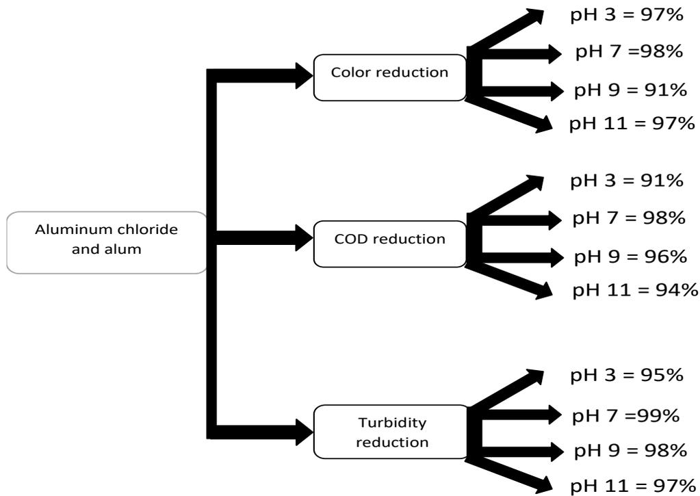
Fig. 5: Percentage reduction of all parameters with treatment T5 at different pH
