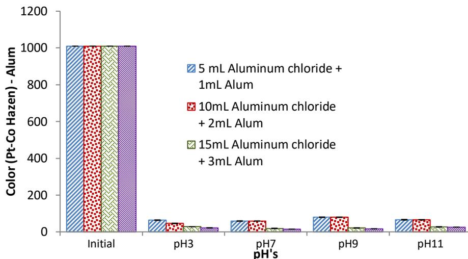
Fig. 2: Color reduction at varying pH by increasing the dose
