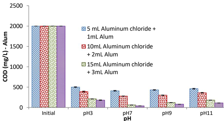
Fig. 3: COD reduction at varying pH by increasing the dose
