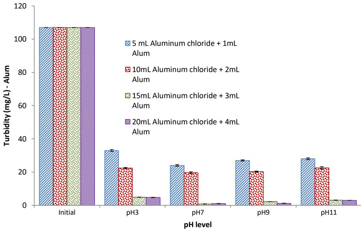
Fig. 4: Turbidity reduction at varying pH by increasing the dose
