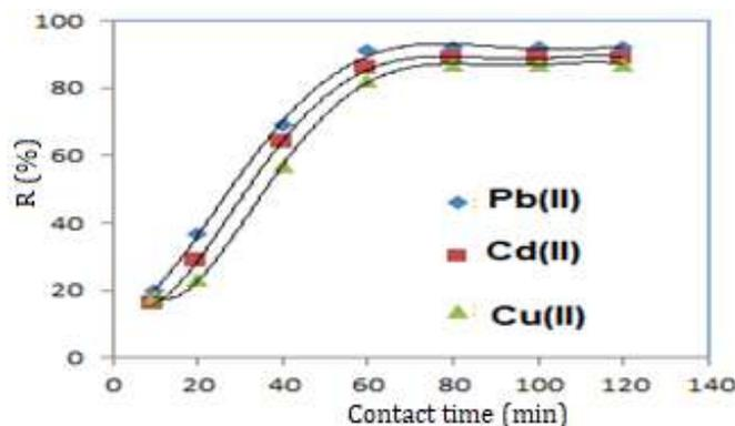
**Fig. 4:** Effect of contact time on the percent removal metal ions by composites. T = 303 K; C<sub>0</sub> = 40 mg/L; pH = 6.0
