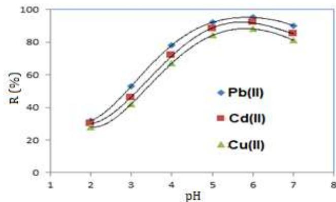
**Fig. 3:** Effect of pH solution on the percent removal metal ions by composites. T = 303 K; C<sub>0</sub> = 40 mg/L; pH = 6.0
