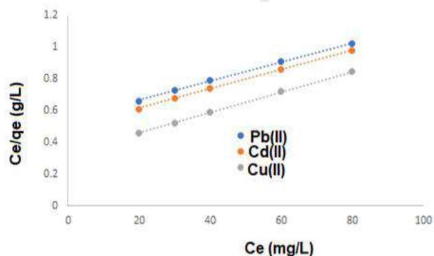
**Fig. 5:** Langmuir isotherm for Pb(II), Cd(II) and Cu(II) ions onto composites
