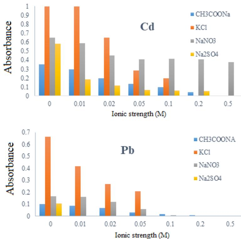
**Fig. 6:** Effect of foreign ions on absorption spectra of Cd(II) and Pb(II) complexes in mixed solvent of water: isopropanol (3:7)
