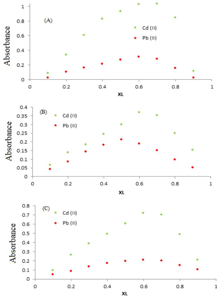
**Fig. 7:** Determination of the metal: reagent ratio of Cd(II) and Pb(II) with murexide complexes using continuous variation method at various mixed solvent ratios
