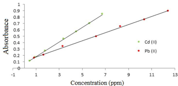
**Fig. 8:** Calibration graph of Cd(II) and Pb(II)
