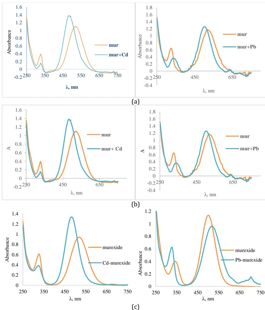
**Fig. 2:** Absorption spectra of Cd(II) and Pb(II) complexes in three different mixed solvents of water: isopropanol; (a) 8:2 (b) 6:4 (c) 3:7
