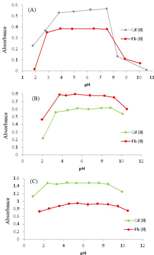
**Fig. 3:** Absorption spectra of Cd(II) and Pb(II) complexes in three different mixed solvents of water: isopropanol; (a) 8:2 (b) 6:4 (c) 3:7
