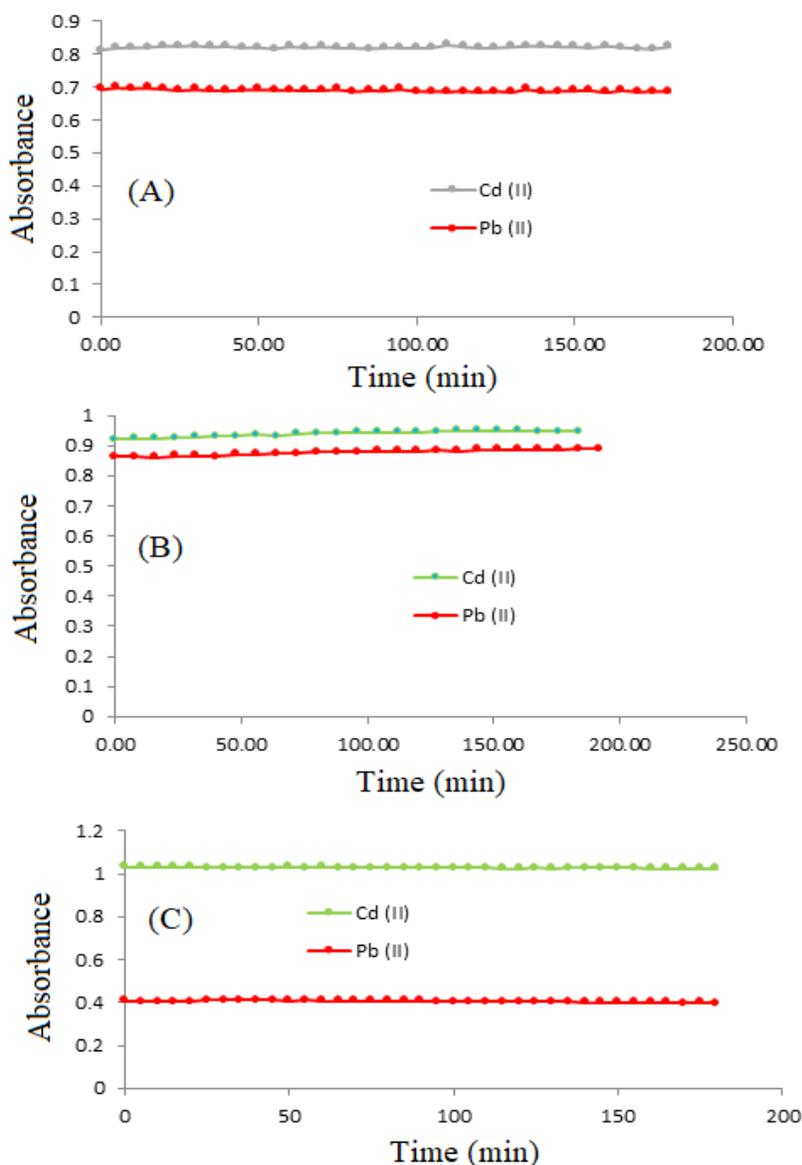
**Fig. 5:** Effect of time on absorption spectra of  $\text{Cd(II)}$  and  $\text{Pb(II)}$  complexes in three different mixed solvents of water: isopropanol; (a) 8:2 (b) 6:4 (c) 3:7
