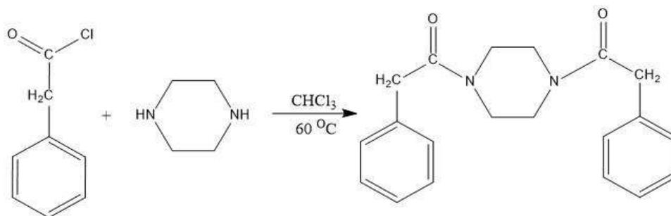
**Scheme 1:** Synthesis of 2-phenyl-1-(4-phenylacetyl-piperazin-1-yl) ethanone (L)
