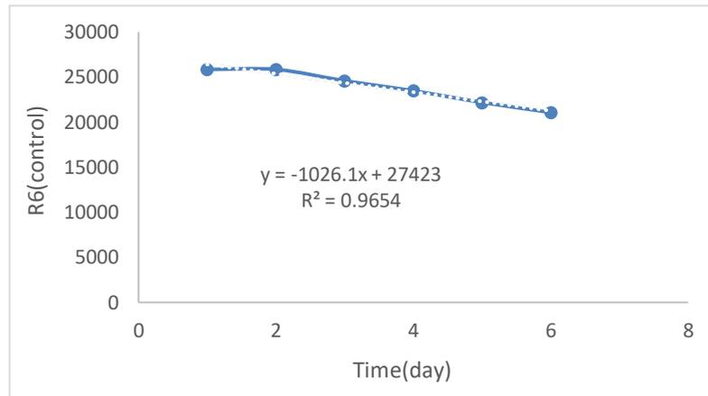
Fig. 6: TPH concentration versus time for R6 (control)
