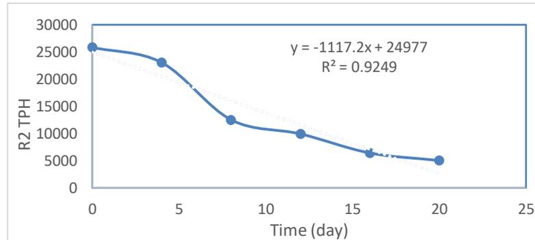
**Fig. 2:** TPH concentration versus time for R<sub>2</sub> (40 g)
