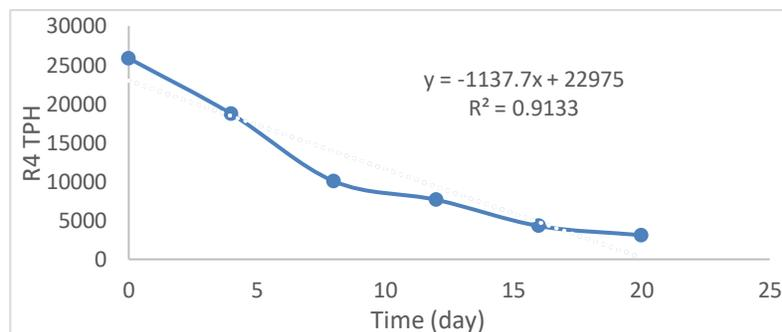
**Fig. 4:** TPH Concentration versus time for R<sub>4</sub> (80 g)
