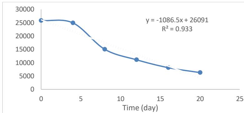
**Fig. 1:** TPH concentration versus time for R<sub>1</sub>(20 g). A-axis = R<sub>1</sub> TPH
