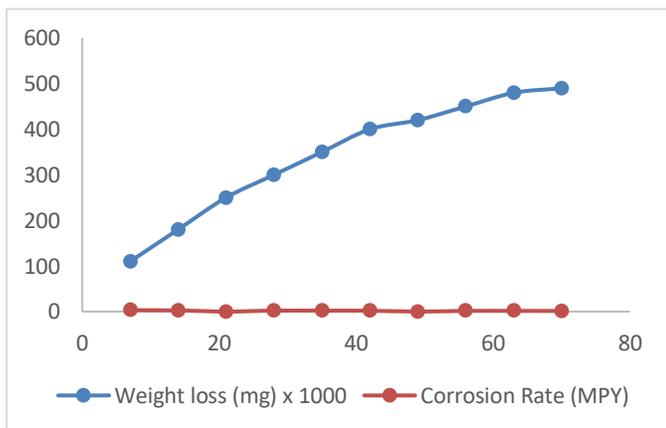
**Fig. 3:** Plot of relationship between weight loss and corrosion rate in a fresh water environment
