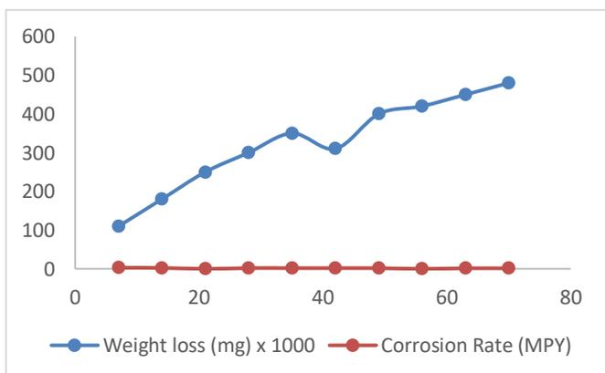
**Fig. 4:** Plot of relationship between weight loss and corrosion rate in an alkaline environment
