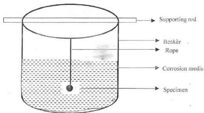
**Fig. 1:** Corrosion medium and set-up
