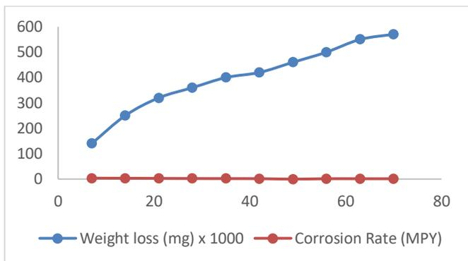
**Fig. 2:** Plot of relationship between weight loss and corrosion rate in a sea water environment
