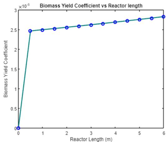
**Fig. 4:** Biomass yield coefficient versus reactor length
