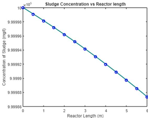
**Fig. 1:** Sludge substrate concentration versus reactor length
