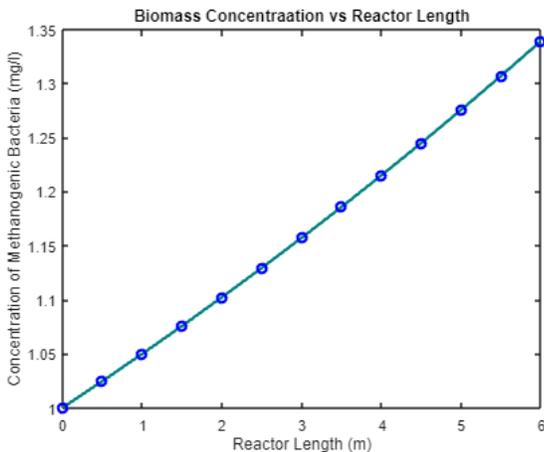
**Fig. 2:** Biomass concentration versus reactor length
